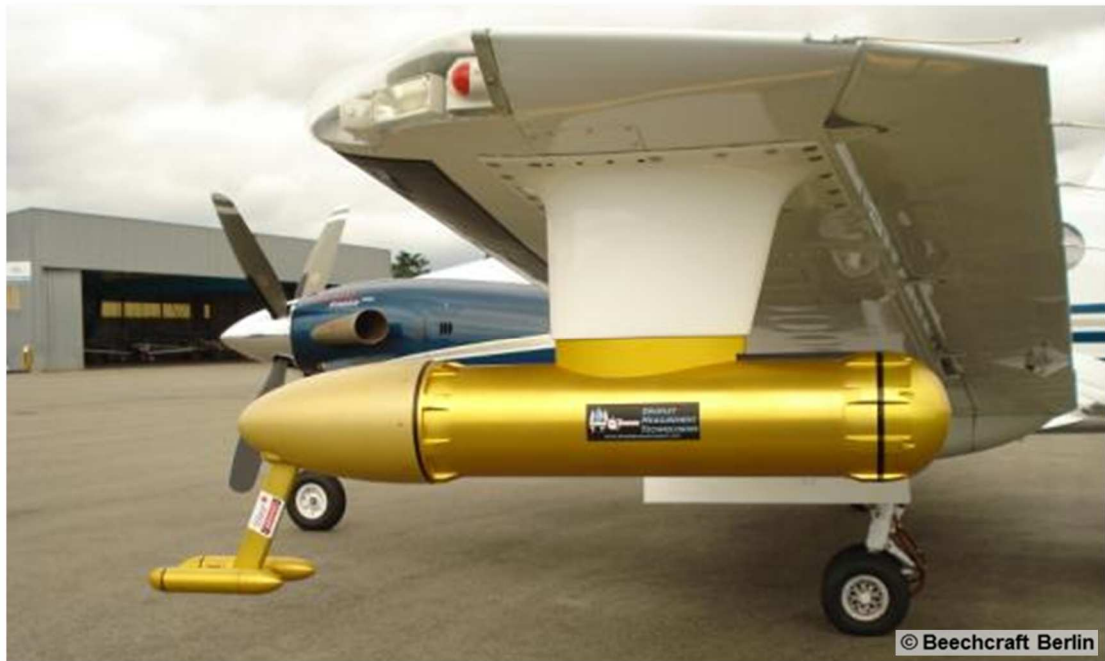
King Air B200 equipped weather research system CAPS (L/H)
