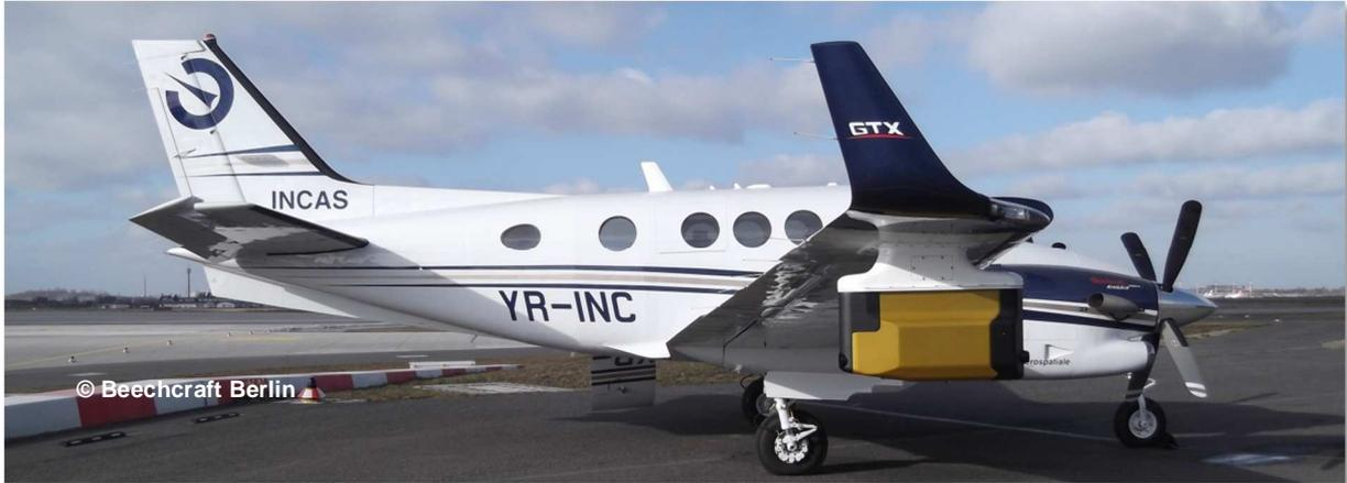
The King Air C90GTi is modified to an airborne laboratory for atmospheric environmental research missions as well as laser scanning for 3D geo-referencing application. Two configurations are currently operating:
