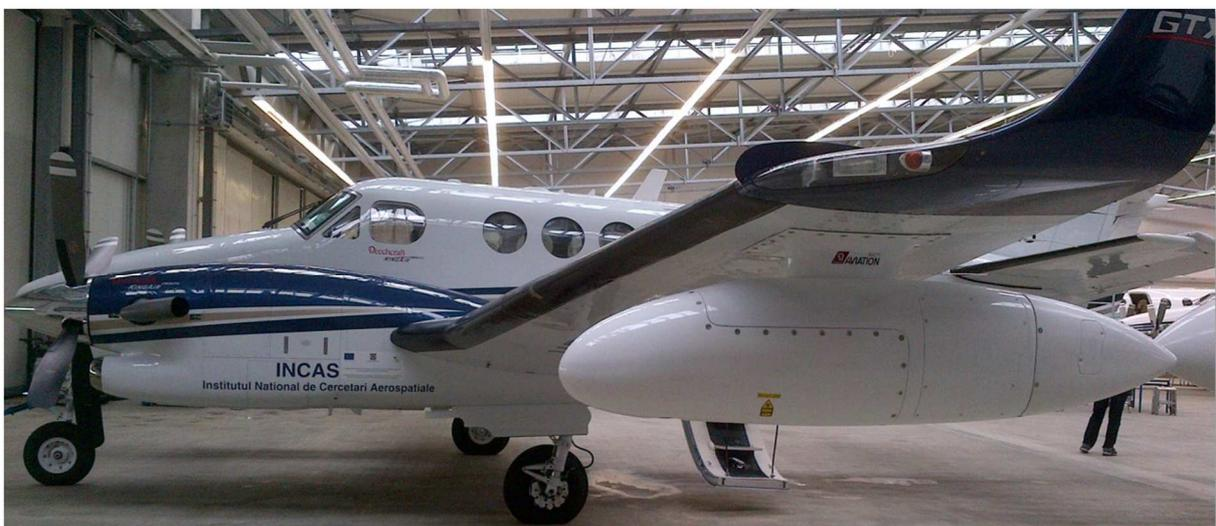
LIDAR and Mission systems inside external multi-purpose pod
